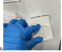
9. Stack no more than 20 petrifilm plates together and place in an incubator at 35° Celsius for 24-48 hours. 10. Clean and sanitize the workstation after plating using a 10% bleach solution.
