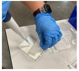
8. Allow the petrifilm to sit for 1 minute after plating before using a plate spreader to apply slight pressure on top of the plastic cover to remove all air bubbles captured under the film.
