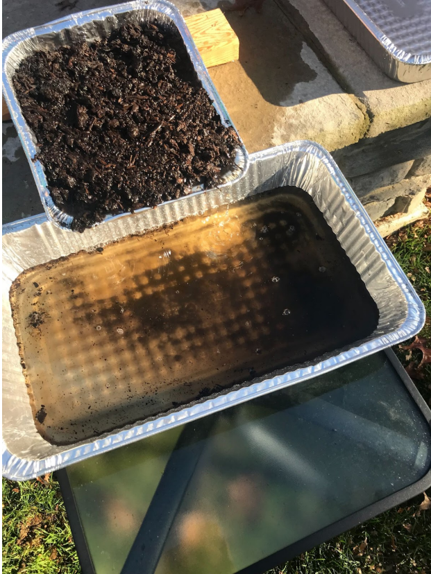
Run off from tray 1 (conventional, no cover crop)
